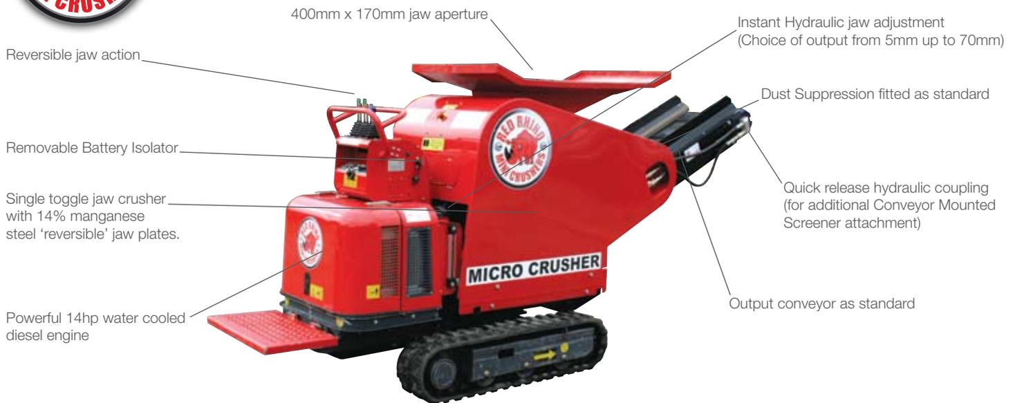
**Description:** Single toggle jaw crusher with jaw aperture of 400mm x 170mm – the only small crusher to accept a full UK kerbstone. The 4000 series is 775mm wide and can travel through doorways, into rear gardens, and enter sites where access and space is restricted. Hydraulically adjustable jaws allow for the adjustment of output product size, ranging from a choice of 5mm up to 70mm.
